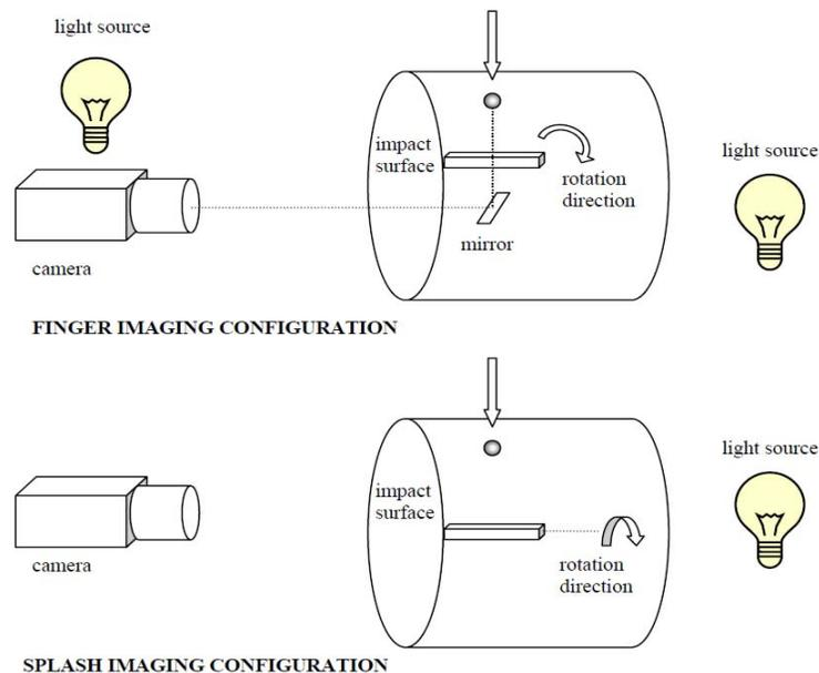
**Figure 1.** Camera and lighting configurations for splash (lateral) and finger (vertical) imaging.
