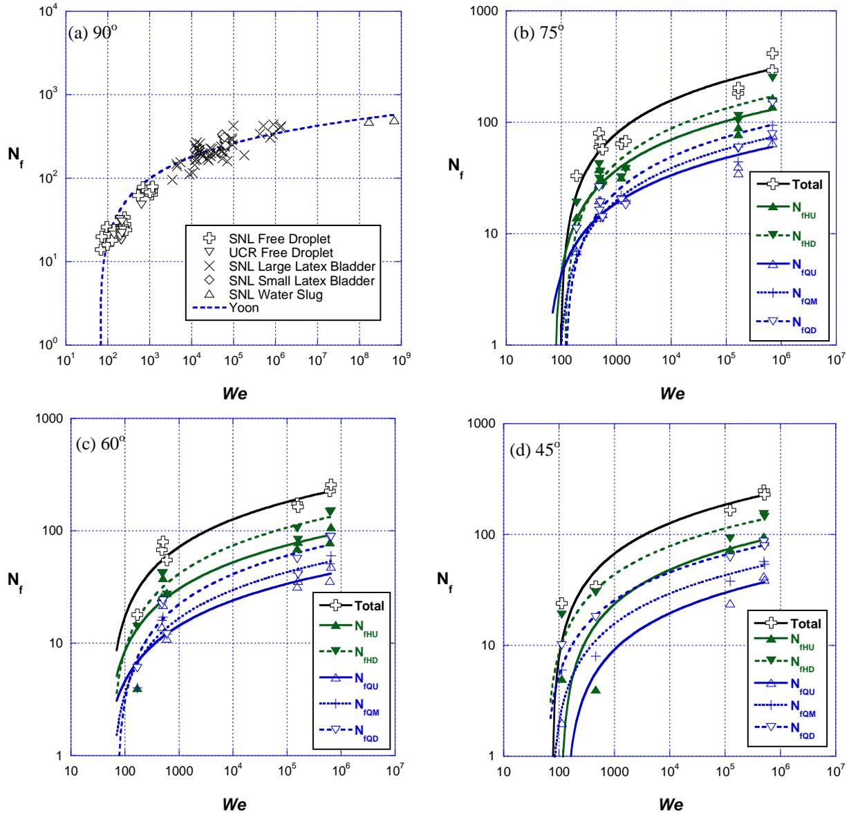
**Figure 5.** Number of fingers ( $N_f$ ) vs.  $We$  at (a) 90°, (b) 75°, (c) 60°, and (d) 45° impact angles for water impacts. Results are from the Sandia small droplet tests, UCR pressure vessel tests at 1 atm, and the Sandia drop tower tests.
