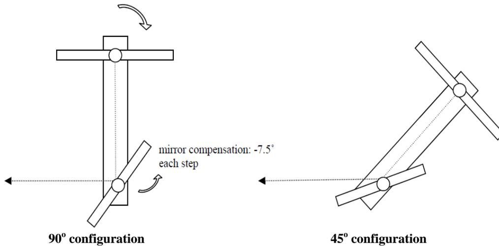
**Figure 2.** Impact surface and mirror configurations for finger imaging.
