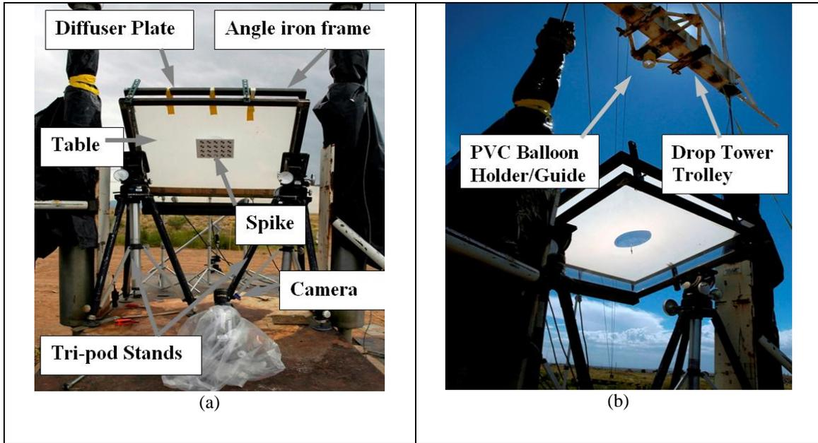
Figure 3. Experimental setup for large scale impact testing.
