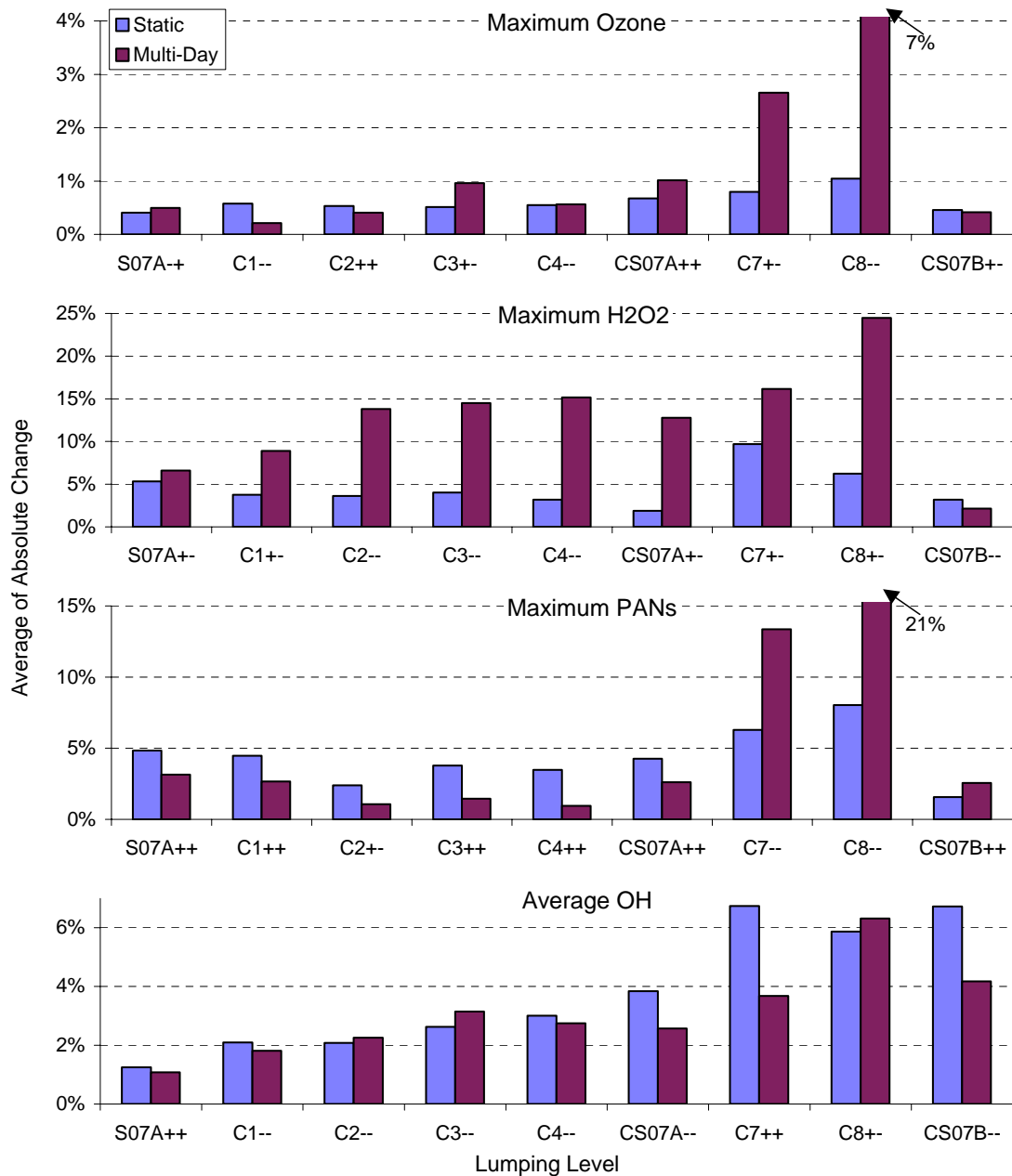
Figure 4. Average changes for maximum O 3 , H 2 O 2 , PANs and average OH for the static and multi-day ROG - NO x test calculations, relative to the uncondensed SAPRC-07 mechanism. "A" = uncondensed mechanism using the SAPRC-99 peroxy radical operators, C1 ... C8 = condensed mechanisms. C6B = C6 mechanism using SAPRC-07 peroxy radical operators (see Table 1). The signs after lumping level indicate the sign for the average differences for the static and multi-day scenarios, respectively.
