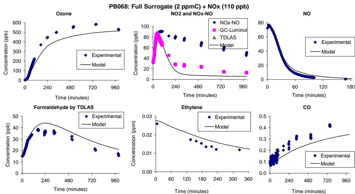
Figure 1. Selected experimental and model calculation results of the photochemical smog simulation experiment carried out at CE-CERT for the IMP collaborators
