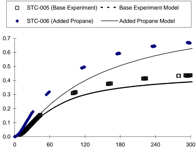
Figure 4. Experimental and calculated concentration-time plots for the base case and the added propane surrogate-NO<sub>x</sub> experiments
