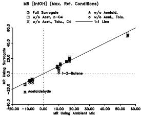
Figure 2. Plots of calculated mechanistic reactivities of selected species in maximum reactivity chamber experiments using various ROG surrogates, against those for similar experiments using the ambient ROG Mixture.
