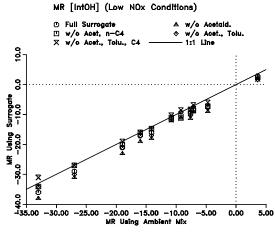
Figure 4. Plots of calculated mechanistic reactivities of selected species in  $\mathrm{NO}_x$ -limited chamber experiments using various ROG surrogates, against those for similar experiments using the ambient ROG mixture.
