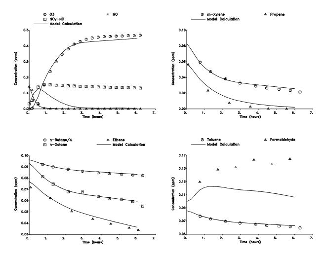
Figure 25. Concentration - time plots for selected species in the base case low  $\mathrm{NO}_{\mathrm{x}}$  lumped surrogate run DTC032A. Results of model calculations are also shown.
