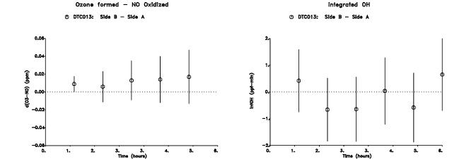
Figure 28. Differences in  $d(O_3-NO)$  and IntOH in a DTC side equivalency test experiment. The "error bars" show the uncertainty ranges as used in the incremental reactivity derivations.
