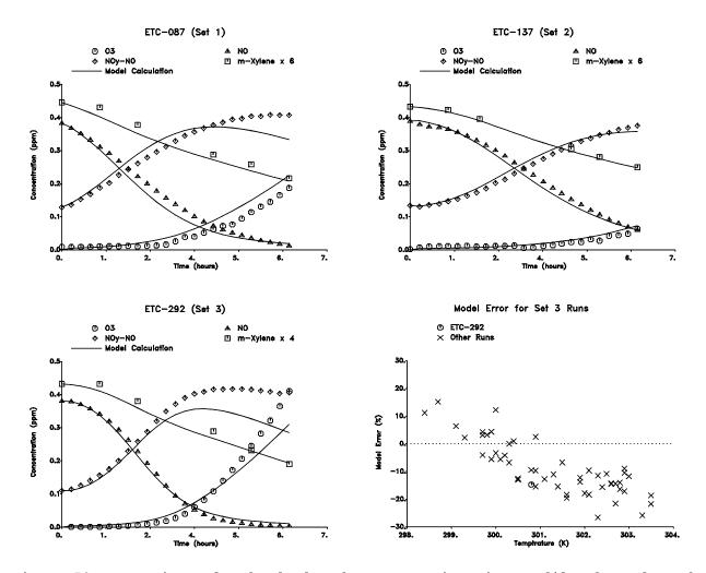
Figure 50. Experimental and calculated concentration-time profiles for selected species in selected Phase I base-case mini-surrogate experiments, and plots of relative errors in model calculations of the Set 3 runs against average temperature.
