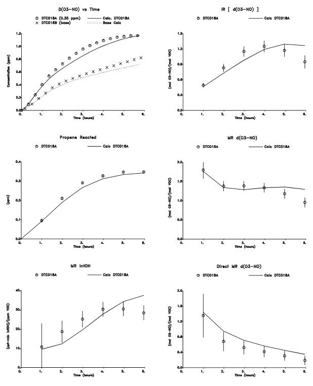
Figure 33. Plots of selected results of the high  $\mathrm{NO}_{\mathrm{x}}$  lumped molecule surrogate reactivity experiment for  $\mathbf{propene}$
