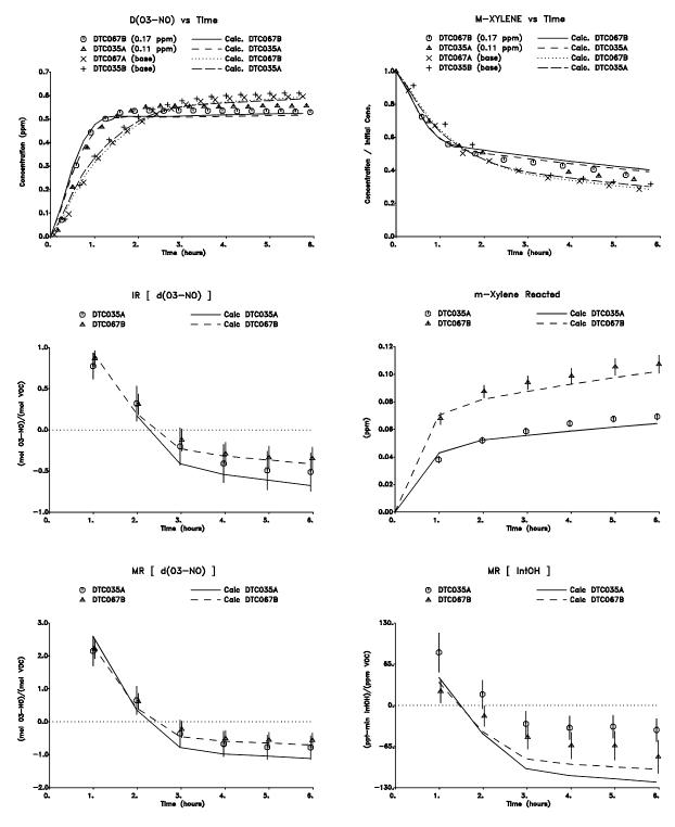
Figure 47. Plots of selected results of the low  ${\rm NO_x}$  lumped molecule surrogate reactivity experiments for  ${\bf m-xylene}$
