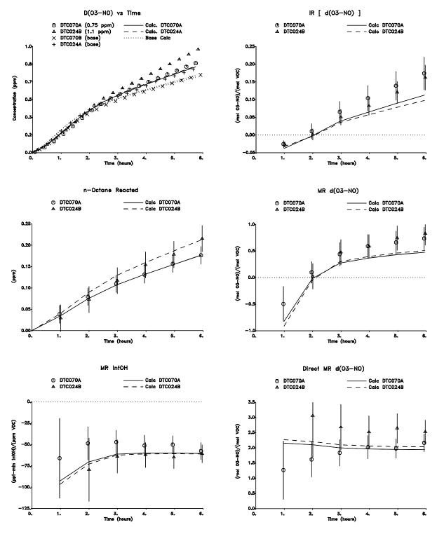
Figure 31. Plots of selected results of the high  $\mathrm{NO}_{\mathrm{x}}$  lumped molecule surrogate reactivity experiments for  $\mathbf{n\text{-}octane}$
