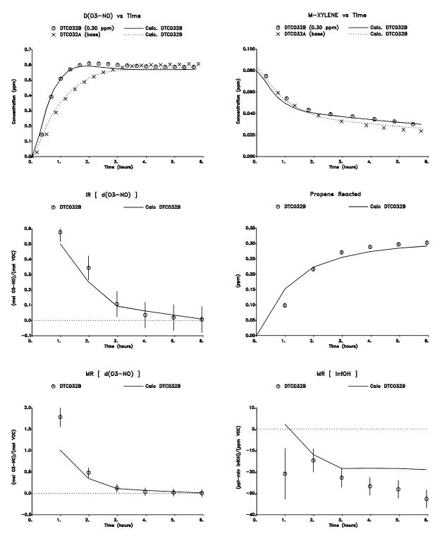
Figure 43. Plots of selected results of the low  $\mathrm{NO}_{\mathrm{x}}$  lumped molecule surrogate reactivity experiment for  $\mathbf{propene}$
