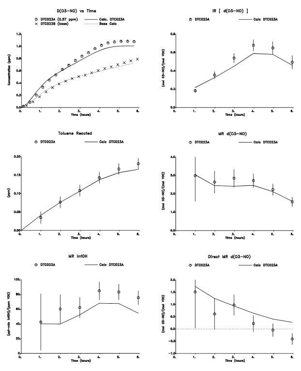
Figure 35. Plots of selected results of the high  $\mathrm{NO}_{\mathrm{x}}$  lumped molecule surrogate reactivity experiment for **toluene**
