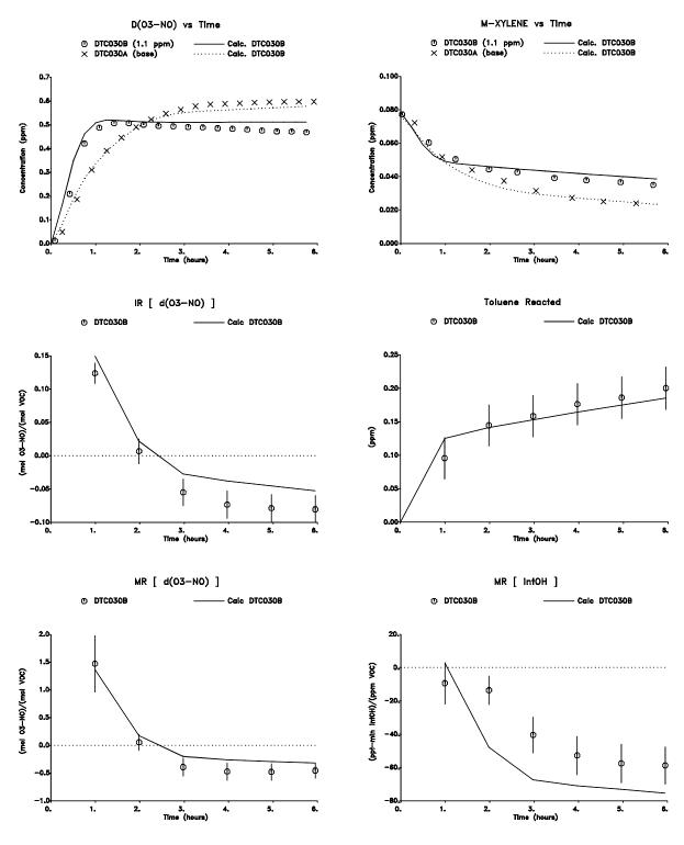
Figure 45. Plots of selected results of the low  $\mathrm{NO}_{\mathrm{x}}$  lumped molecule surrogate reactivity experiment for  $\mathbf{toluene}$
