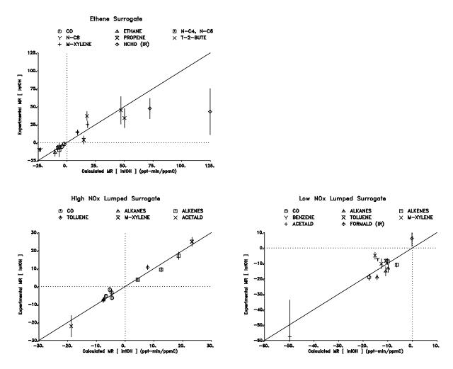
Figure 53. Plots of experimental  $\underline{vs}$  calculated 6-hour IntOH mechanistic reactivities for the various types of reactivity experiments. Note that the reactivities are given on a per-carbon basis.
