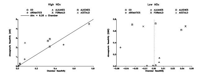
Figure 56. Plots of atmospheric incremental reactivities (carbon basis) against incremental reactivities in the environmental chamber experiments using the lumped surrogate. High  $\mathrm{NO}_{\mathrm{x}}$  chamber reactivities are plotted against atmospheric reactivities in the MIR scale, and low  $\mathrm{NO}_{\mathrm{x}}$  chamber reactivities are plotted against atmospheric reactivities in the low  $\mathrm{NO}_{\mathrm{x}}$  "Equal Benefit Incremental Reactivity" scale.
