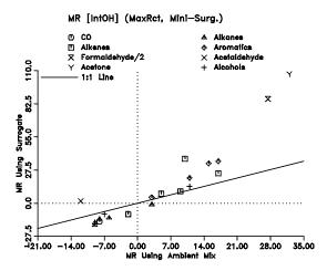
Figure 5. Plots of calculated mechanistic reactivities of selected species in maximum reactivity chamber experiments using the 3-component minisurrogate, against those for similar experiments using the ambient ROG mixture.
