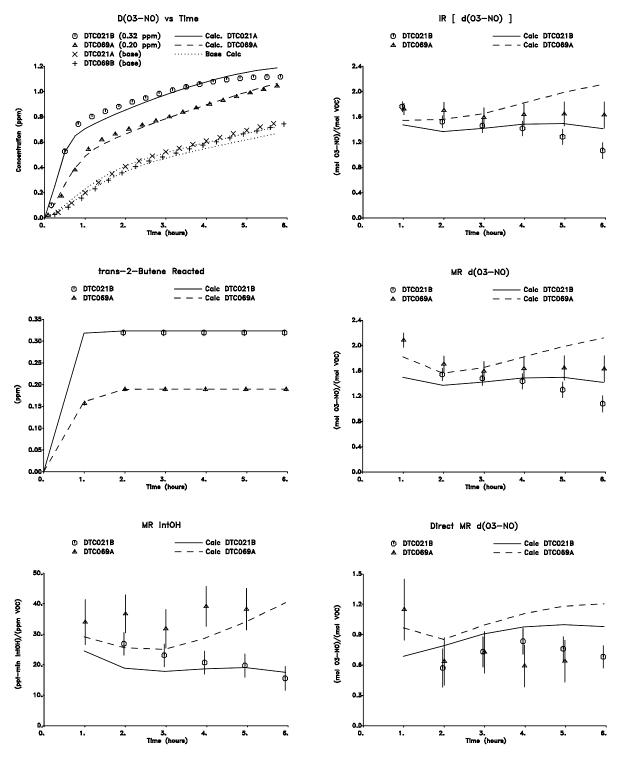
Figure 34. Plots of selected results of the high  ${\rm NO_x}$  lumped molecule surrogate reactivity experiments for  ${\rm \underline{trans}\text{-}2\text{-}Butene}$
