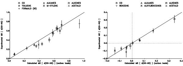
Figure 52. Plots of experimental  $\underline{vs}$  calculated 6-hour  $d(O_3-NO)$  mechanistic reactivities for the various types of reactivity runs. Note that the reactivities are given on a per-carbon basis.
