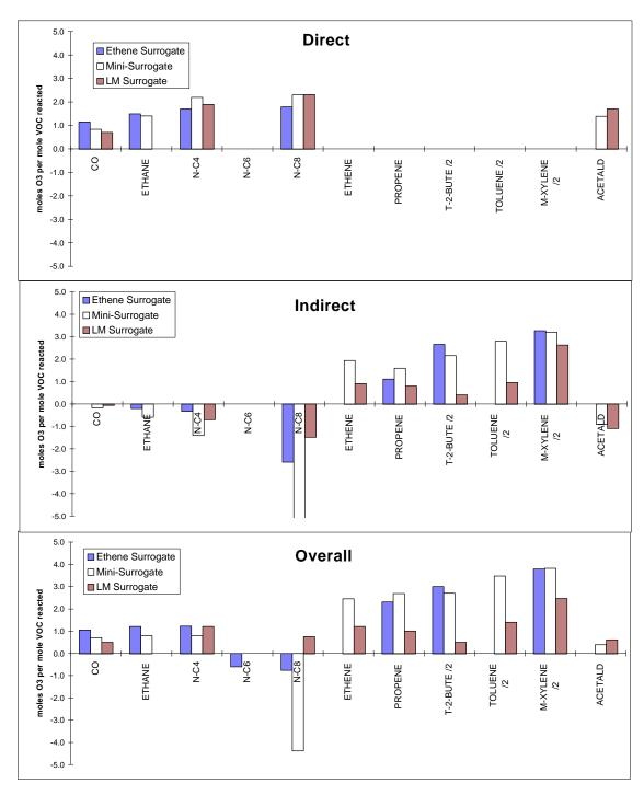
Figure 55. Comparisons of weighed averages of the direct, indirect, and overall mechanistic reactivities for high NOx conditions for the three base ROG surrogates. The averages are of the data on Table 15. The units of the data are moles d(03-N0) per mole VOC reacting.
