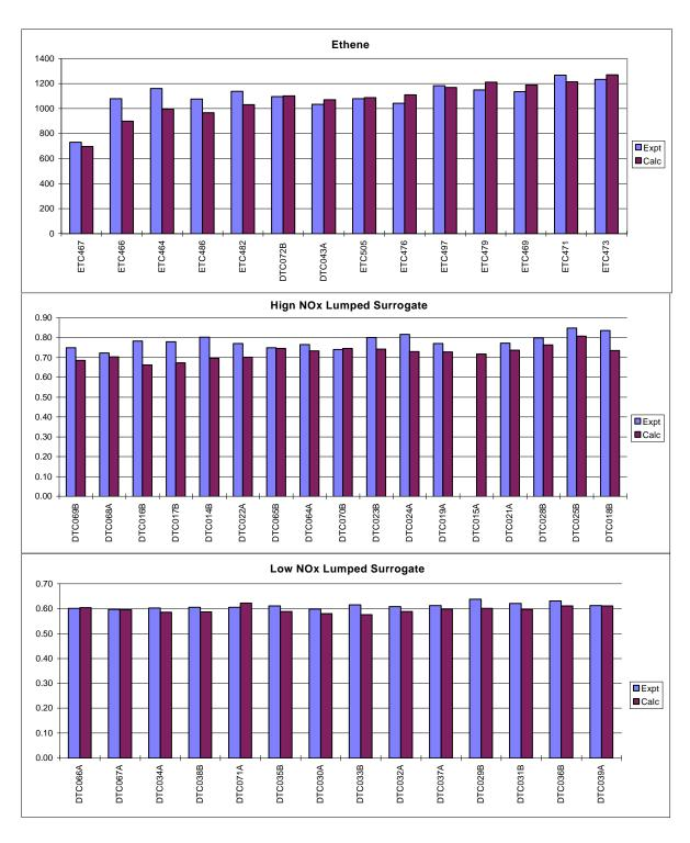
Figure 51. Comparisons of experimental and calculated 6-hour d(03-N0) for the base case experiments. Units are ppm.
