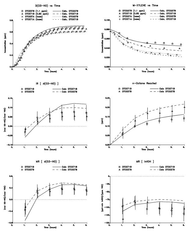
Figure 41. Plots of selected results of the low  $\mathrm{NO}_{\mathrm{x}}$  lumped molecule surrogate reactivity experiments for  $\mathbf{n}\text{-}\mathbf{octane}$
