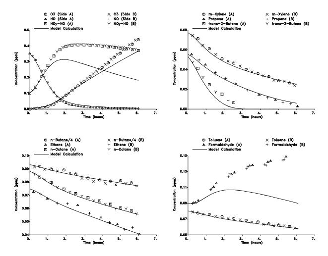
Figure 24. Concentration - time plots for selected species in the base case high  $\mathrm{NO}_{\scriptscriptstyle x}$  lumped surrogate run DTC013. This run is a side equivalency test with the same mixture irriadiated on both sides. Results of model calculations are also shown.
