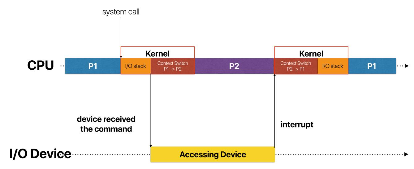
If T<sub>Context</sub> switch P1->P2 + T<sub>Context</sub> switch P2->P1 < T<sub>Accessing</sub> peripherals
