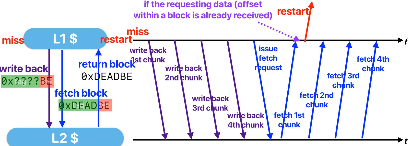
assume the bus between L1/L2 only allows a quarter of the cache block go through it
