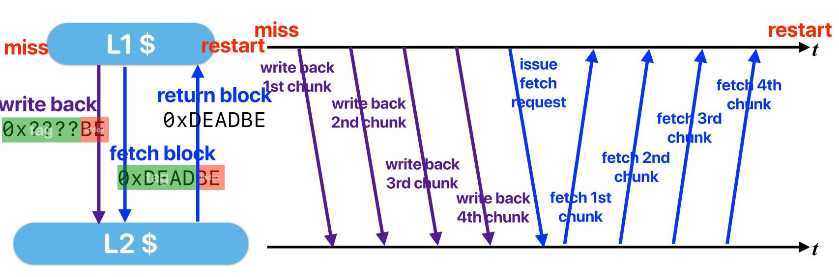
assume the bus between L1/L2 only allows a quarter of the cache block go through it
