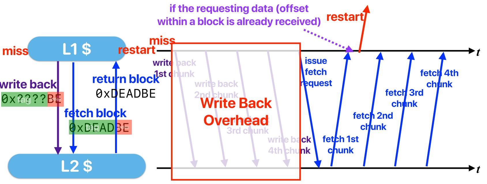
assume the bus between L1/L2 only allows a quarter of the cache block go through it
