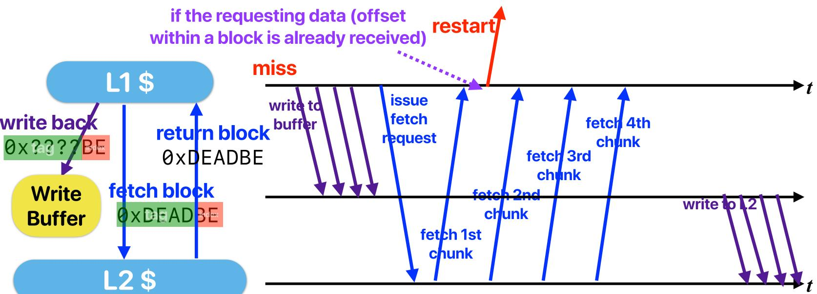
assume the bus between L1/L2 only allows a quarter of the cache block go through it
