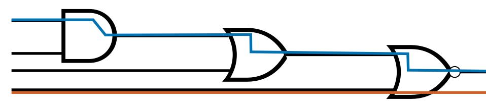
Which path in the above circuit determines the propagation delay of the circuit (assuming the delay of all the gates is the same)?
