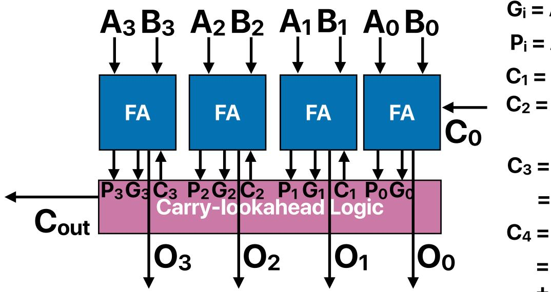
$$\begin{aligned} G_i &= A_i B_i \\ P_i &= A_i XOR B_i \\ C_1 &= G_0 + P_0 C_0 \\ C_2 &= G_1 + P_1 C_1 = G_1 + P_1 (G_0 + P_0 C_0) \\ &= G_1 + P_1 G_0 + P_1 P_0 C_0 \\ C_3 &= G_2 + P_2 C_2 \\ &= G_2 + P_2 G_1 + P_2 P_1 G_0 + P_2 P_1 P_0 C_0 \\ C_4 &= G_3 + P_3 C_3 \\ &= G_3 + P_3 G_2 + P_3 P_2 G_1 + P_3 P_2 P_1 G_0 \\ &+ P_3 P_2 P_1 P_0 C_0 \end{aligned}$$
