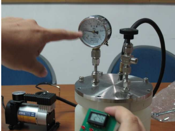
Figure B17: Comparing pressure readings
