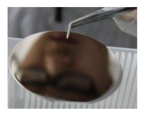
After a week of baking, washing, drying, and testing the silicon wafers for consistency, they are put into a big oven and coated with platinum.
