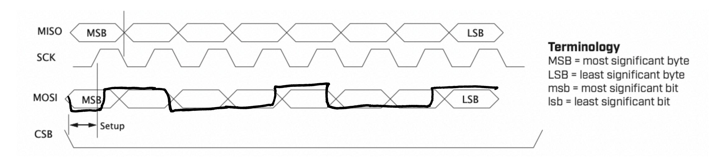
Let's look at real timing diagrams from an encoder with SPI interface
