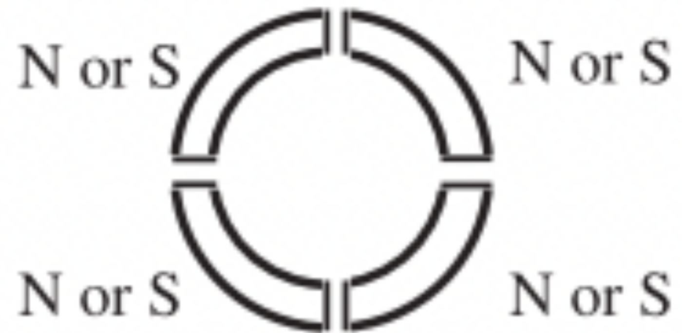
stator with reversible polarity poles
