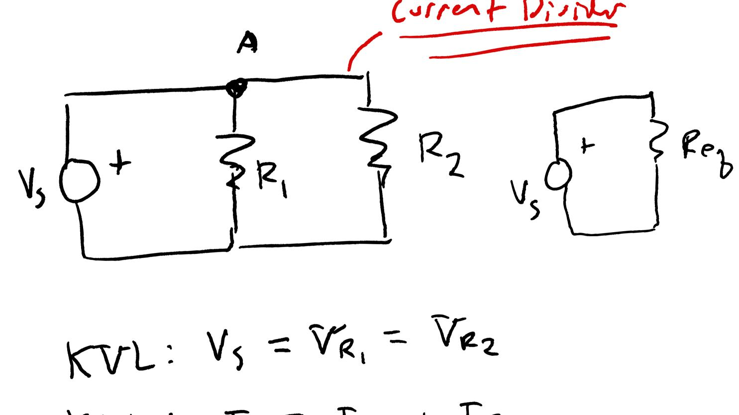
$$KVL: V_{S} = V_{R_{1}} = V_{R_{2}}$$
