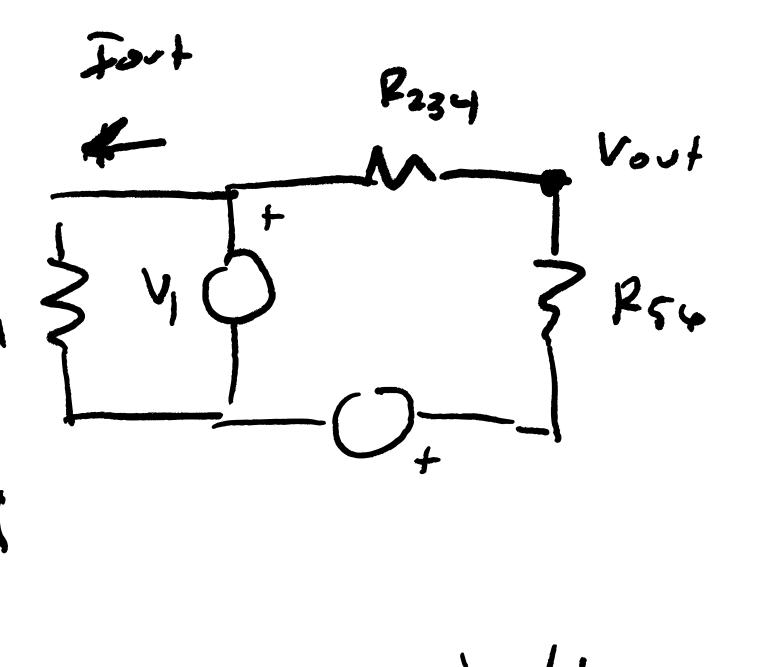
$$R_{234} = \frac{(R_2 + R_4) \cdot R_3}{R_2 + R_3 + R_4}$$
