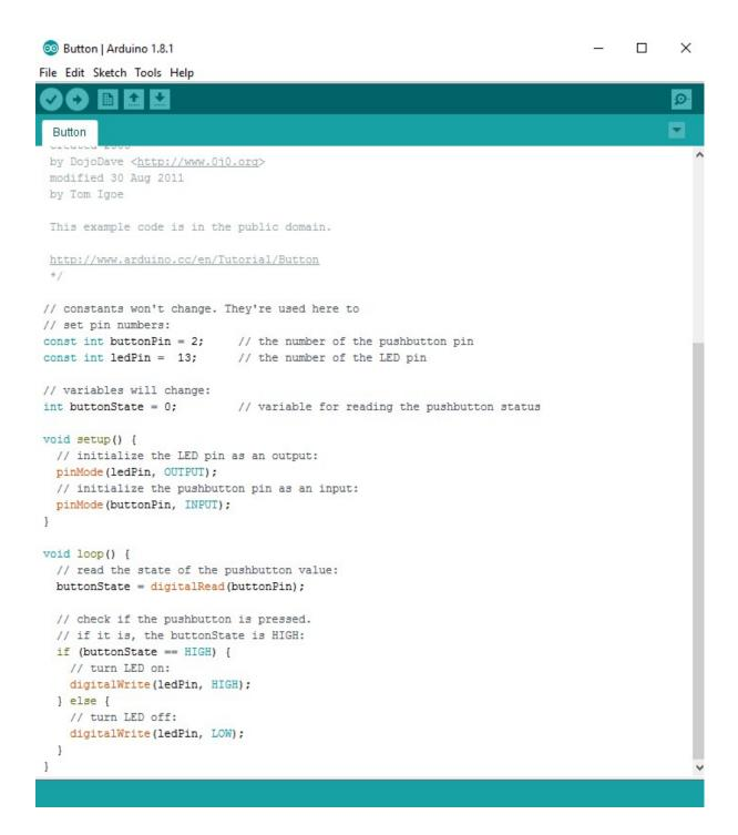
Next, you need to click on the verify button (check mark) that's located in the top left of the IDE box. Once it says "Done Compiling" you are ready to upload it. Click the upload button (forward arrow) to send the program to the Arduino board.
