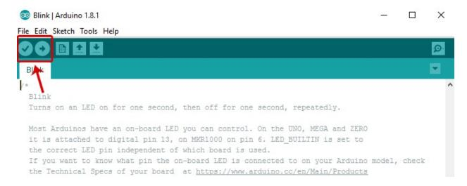
The built-in LEDs on the Arduino board will flash rapidly for a few seconds and then the program will execute. If everything went correctly, the LED on the breadboard should turn on for a second and then off for a second and continue in a loop.
