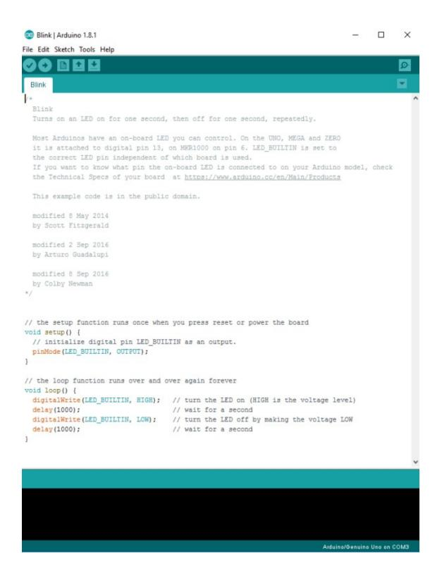
Next, you need to click on the verify button (check mark) that's located in the top left of the IDE box. This will compile the sketch and look for errors. Once it says "Done Compiling" you are ready to upload it. Click the upload button (forward arrow) to send the program to the Arduino board.
