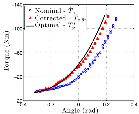
**Fig. 16** Experimental validation of cam elastic response. The circles represent the experimental data points for the nominal case. The triangles are experimental data points with a 3 mm shim added to the device.
