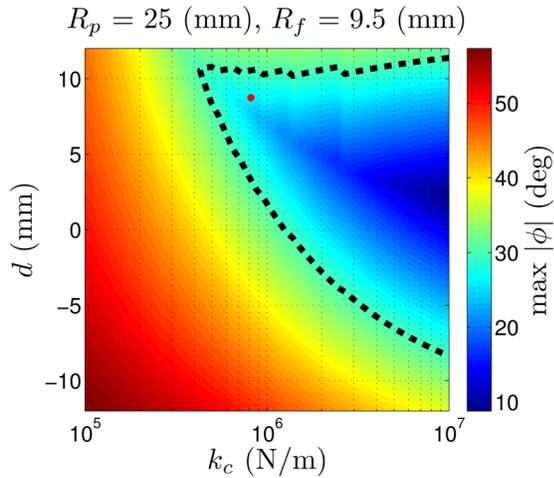
**Fig. 12** Pressure angle  $\phi$  for different follower stiffness  $k_c$  and eccentricity  $d$ . Dotted line denotes maximum allowable pressure angle,  $\max|\phi| = 30$  deg. The red dot denotes the prototype configuration.
