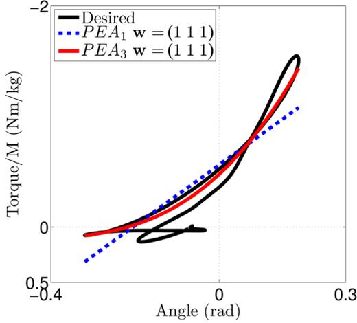
**Fig. 8 The nonamputee ankle stiffness characteristics (normalized torque  $T/M$  versus desired angular displacement  $\theta_d$ ) for the entire gait cycle, superimposed with the linear PEA<sub>1</sub> and third-degree nonlinear PEA<sub>3</sub> stiffness profiles**
