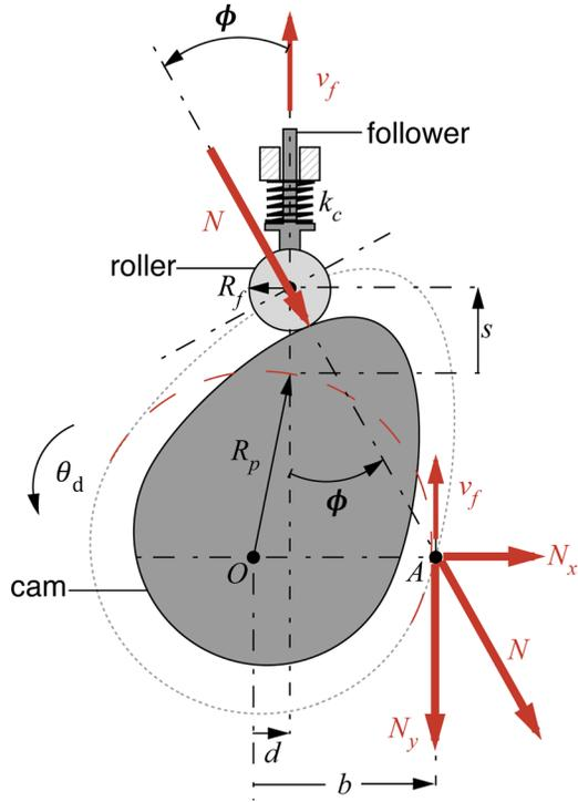
**Fig. 11** Schematic of the cam-follower mechanism adapted from Ref. [33]. The cam rotates about point  $O$  (the center of the prime radius  $R_p$ ), which is  $d$  away from the line of action of the cam follower, whose displacement is  $s$  and velocity is  $v_f$ . The pressure angle  $\phi$  is the angle between the normal force  $N$  and the follower's line of action. The instant center of rotation is  $A$ , which is  $b$  away from the center of rotation  $O$ .
