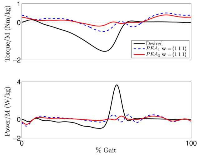
**Fig. 9 Comparison of normalized actuator torque  $T_a/M$  and power  $P_a/M$  for optimal linear PEA<sub>1</sub> with those for the optimal, third-degree nonlinear PEA<sub>3</sub> with  $w = [1\ 1\ 1]$**
