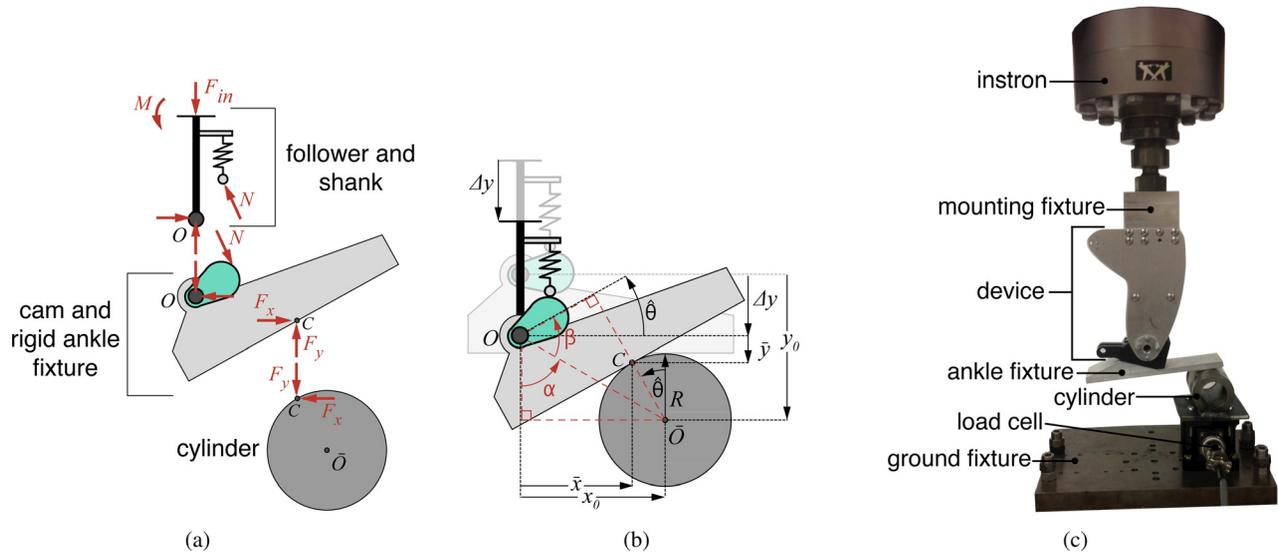
**Fig. 15** Images detailing the static loading experiment. (a) Free body diagram of static loading experiment. (b) Schematic of static loading experiment illustrating the geometry and the angular displacement  $\hat{\theta}$ , caused by input displacement  $\Delta y$ . (c) Image of experimental setup.
