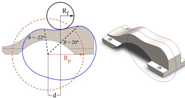
**Fig. 13** Cam prototype for PEA<sub>3</sub> with parameters in Table 3. The black dashed lines represent the boundaries of the functional area:  $-22$  deg for plantarflexion and  $20$  deg for dorsiflexion.
