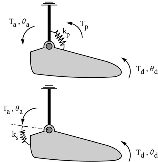
**Fig. 4** Schematic representations of 1DOF powered ankle configurations. (Top) The PEA configuration is characterized by an ideal torque source  $T_a$  in parallel with a rotational passive component. The parallel component generates a torque  $T_p$  as a function of the angular displacement  $\theta_a$ . (Bottom) The SEA configuration consists of an ideal torque source  $T_a$  in series with a rotational passive component.
