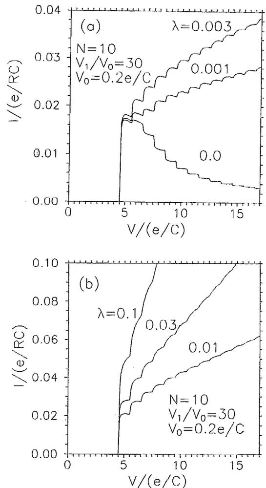
FIG. 3. The dc  $I$ - $V$  curves of a "slim" (small cross section) superlattice for several values of the parameter  $\lambda$ . Such superlattices exhibit strong single-electron charging effects: the Coulomb blockade of tunneling at  $V < V_t = (N-1)e/2C$ , and a structure with the period  $\Delta V = e/C$  due to quantization of electric charge of the high-field domains at  $V > V_t$ .
