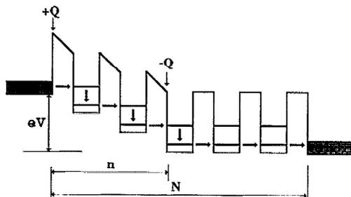
FIG. 2. Schematic band diagram of a superlattice with a high-field domain embracing  $n$  tunnel barriers (of the total number  $N$ ).
