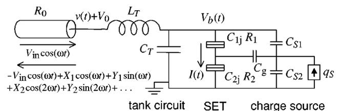
FIG. 1. Schematic of the rf-SET.
