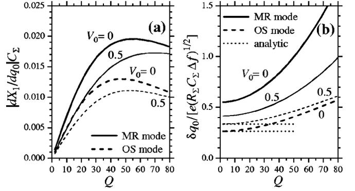
FIG. 2. (a) Rf-SET response and (b) sensitivity as functions of the  $Q$ -factor in the maximum response (MR) and optimal sensitivity (OS) modes.  $T = 0.01 e^2/C_\Sigma$ ,  $R_\Sigma/R_0 = 2000$ ,  $\omega = \omega_0$ .
