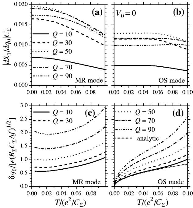
FIG. 3. Dependence of (a) and (b) rf-SET response and (c) and (d) sensitivity on temperature  $T$  in the MR and OS modes for several  $Q$ -factors.  $V_0=0$ ,  $R_\Sigma/R_0=2000$ , and  $\omega=\omega_0$ .
