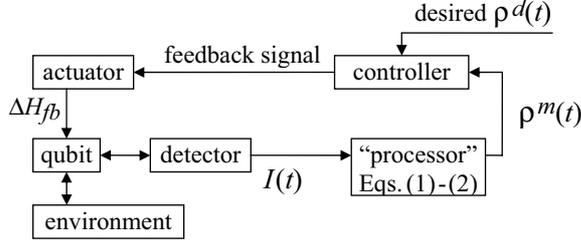
**Figure 1.** Schematic of the quantum feedback loop. By comparing the monitored qubit state  $\rho^m$  with the desired state  $\rho^d$ , a certain algorithm (controller) produces the feedback signal which changes the qubit tunneling amplitude  $H_{fb}$  in order to reduce the difference between  $\rho^m$  and  $\rho^d$ .
