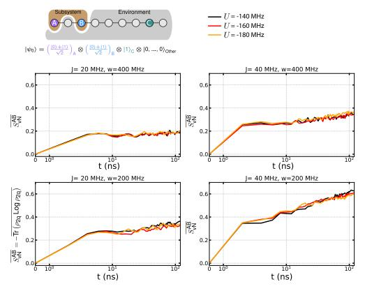
Figure S19: Disorder averaged von Neumann entropy vs. U for selected couplings and disorder magnitudes. The von Neumann entropy observed in the experiment is predicted to be insensitive to the precise value of U.
