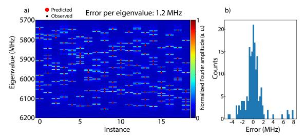
Figure S3: Many-body Ramsey calibration data for 9 qubit randomly generated Hamiltonians. (a) Fourier data for 18 instances of randomly generated Hamiltonians overlayed with the control model predictions of the eigenvalues. (b) A histogram of the difference between the control model predicted eigenvalues and the experimentally observed peaks.
