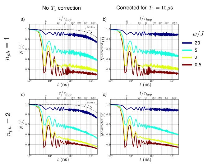
Figure S5: Transport Measurements: Decoherence Effects. (a) The raw disorder averaged transport data for  $n_{ph} = 1$  (b) The data from (a) corrected for a simple energy relaxation model  $\overline{N^{corrected}(t)} = \overline{N(t)}/e^{(-t/10\mu s)}$ . (c) The raw disorder averaged transport data for  $n_{ph} = 2$ . (d) The disorder averaged transport data with  $T_1$  correction.
