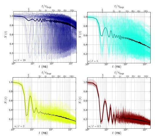
Figure S4: Transport measurement instances. Instances of N(t) for the transport protocol of main text Fig. 2 prior to disorder averaging. Data shown here is for  $J = 40 \,\text{MHz}$  and  $n_{ph} = 2$ .
