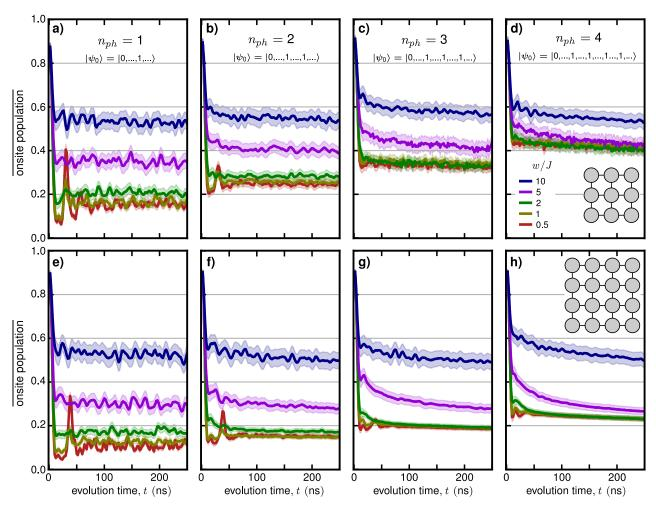
Figure S13: Extended data for onsite population of 2D arrays. (a-d) Onsite population for  $n_{ph} = 1, 2, 3, 4$  on a 3x3 array of qubits. (e-h) Onsite population for  $n_{ph} = 1, 2, 3, 4$  on a 4x4 array of qubits.
