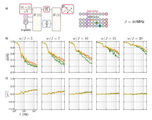
Figure S10: Interferometric Protocols: Extended Data. (a) Spin and DEER echo pulse sequences. We the blue outline indicates the position of the DEER echo pulse, and the position of an additional excitation is indicated in purple. (b) purity of the single qubit density matrix after the spin echo (dashed red lines) and DEER echo (solid lines) experiments. (c)  $\langle \sigma^z \rangle$  monitored over the echo experiments.
