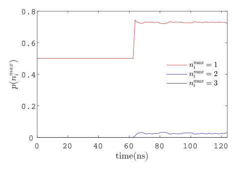
Figure S8: Numerical estimate of the occupation of higher transmon levels during the DEER echo protocol. Calculation shown here for the one, two, and three excitation states
