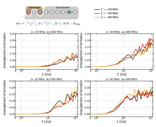
Figure S20: Disorder averaged entanglement of formation vs. U for selected couplings and disorder magnitudes. The entanglement of formation observed in the experiment is predicted to be insensitive to the precise value of U.
