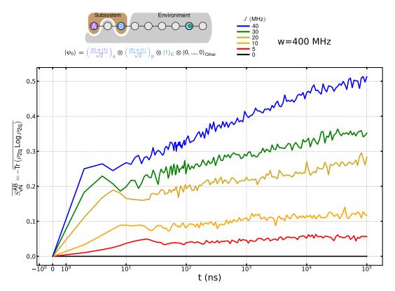
Figure S18: Entropy comparison with numerics. Numerics to longer times than are accessible in the experiment illustrating the predicted logarithmic growth of entanglement for our system.
