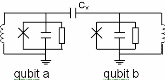
Pseudospin measurement along arbitrary axis  $(\vec{a}, \vec{a}', \vec{b}, \vec{b}')$  is realized by rotation (microwave) + measurement along z-axis.
