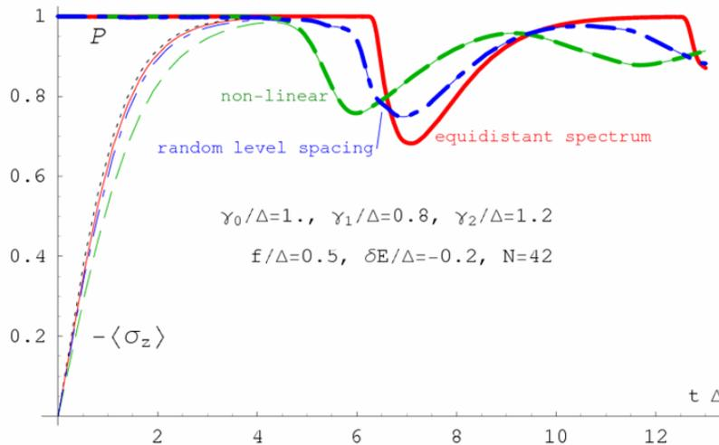
**Better model:** tunneling into discrete levels + decoherence (in the second well and inter-well)
