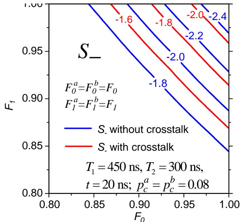
Equal errors and crosstalk make preferable measurement of *positive*  $S$
