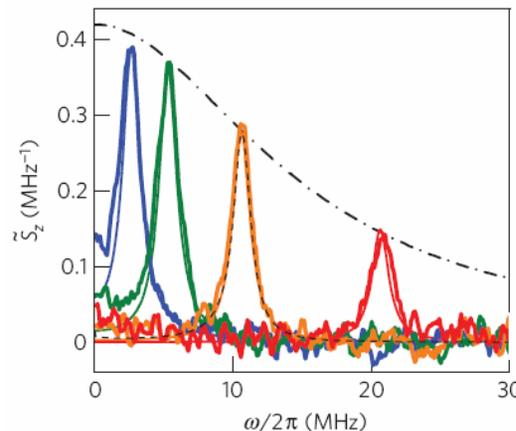
Quantum efficiency limits fidelity of quantum feedback (synchronization of persistent Rabi oscillations)
