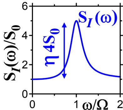
peak height of persistent Rabi oscillations is limited by 4 times noise pedestal (quantum limit); state of the art: 2%
