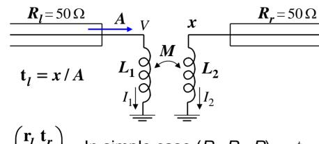
$S = \begin{pmatrix} \mathbf{r}_{l} \ \mathbf{t}_{r} \\ \mathbf{t}_{l} \ \mathbf{r}_{r} \end{pmatrix} \text{ In simple case } (R_{l} = R_{r} = R) \text{ t}$ S-matrix is unitary,  $\mathbf{t}_{r} = \mathbf{t}_{l} = \mathbf{t}, \ \mathbf{r}_{r} = -\mathbf{r}_{l}^{*}(\mathbf{t}/\mathbf{t}^{*})$  $\mathbf{t}/\sqrt{\mathbf{r}_{l}\mathbf{r}_{r}} \text{ is imaginary}$
