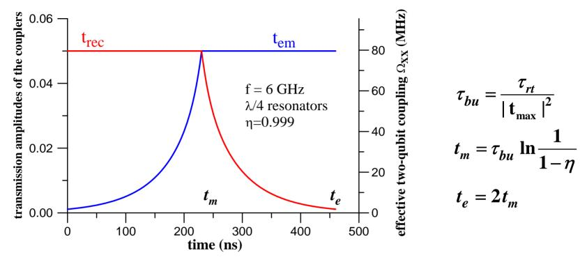
No initial build-up period t<sub>s</sub>. Just <u>pretend</u> the needed amplitude is already in the receiving resonator. Then a fully symmetric procedure.
