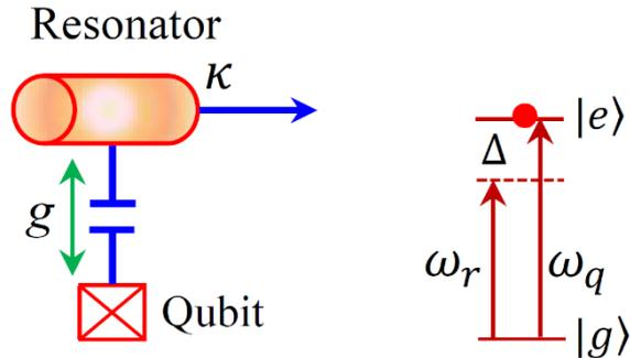
“Usual” Purcell effect: energy relaxation of a qubit via coupling with a leaking resonator
