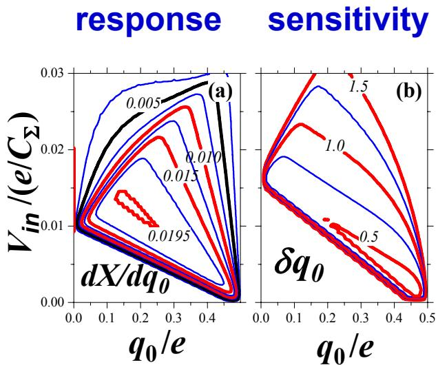
**Optimizations of response and sensitivity are different (rf amplitude is much smaller for optimal sensitivity)**
