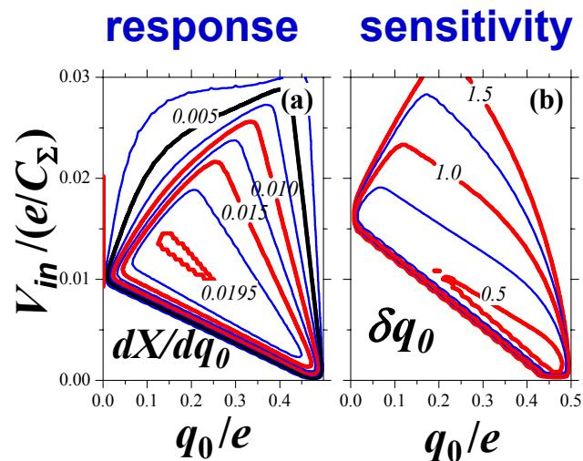
Optimizations of response and sensitivity are different (rf amplitude is much smaller for optimal sensitivity)
