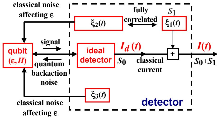
$$\begin{aligned}\frac{d}{dt} \rho_{11} &= -2H \operatorname{Im} \rho_{12} + \rho_{11} \rho_{22} \frac{2\Delta I}{S_I} [I(t) - I_0] \\ \frac{d}{dt} \rho_{12} &= i\tilde{\epsilon} \rho_{12} + iH(\rho_{11} - \rho_{22}) + iK[I(t) - I_0] \\ &\quad + \rho_{12}(\rho_{11} - \rho_{22}) \frac{\Delta I}{S_I} [I(t) - I_0] - \tilde{\gamma} \rho_{12}\end{aligned}$$
