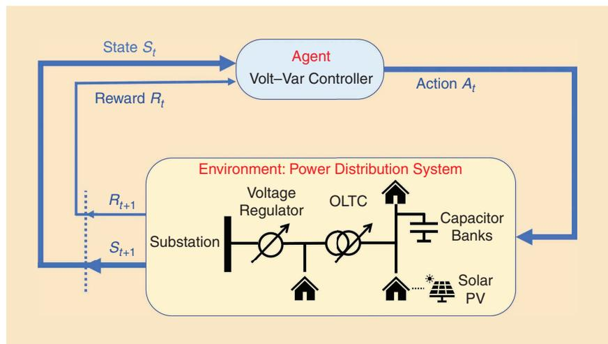
Figure 3. VVC through RL. OLTC: on-load tap changer.
