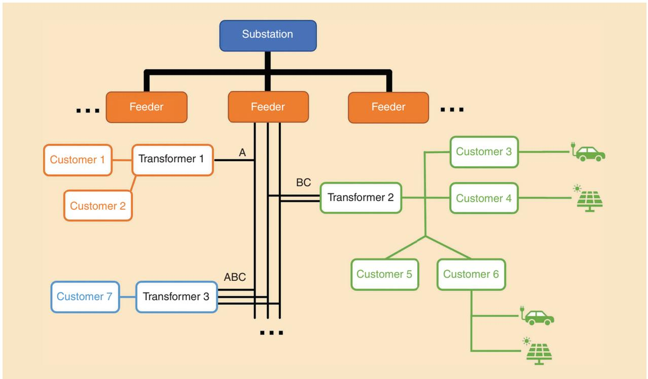
**Figure 1.** A distribution system model with BTM resources.
