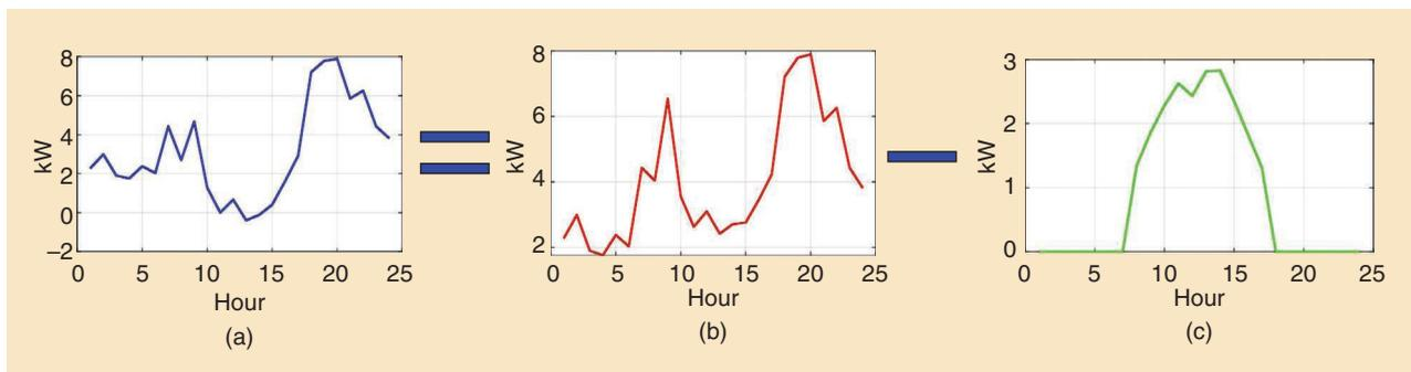
**Figure 2.** The net load disaggregation of a house. The (a) net load equals the (b) load minus (c) solar PV generation.
