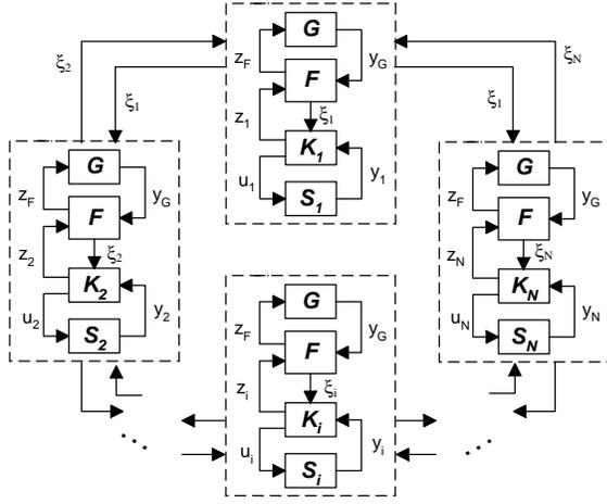
**Figure 1:** The decentralized architecture via the virtual structure approach.
