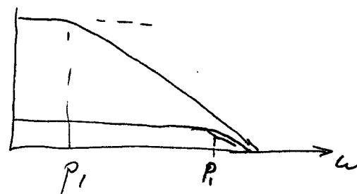
$$(\text{Gain} \cdot \text{Bandwidth})(\omega=0) = \text{const.}$$
