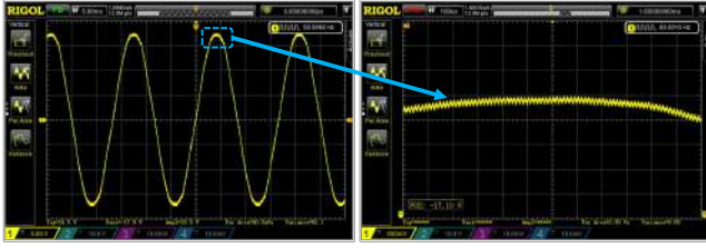
Figure 7: High-frequency voltage ripples at the PDU caused by switching in the server power supply unit.
