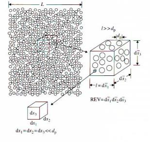
**FIGURE 2.1**The schematic to illustrate the scaling law and the REV for the volumetric average scheme.
