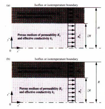
**FIGURE 4.1** Definition sketch: (a) parallel-plate channel, (b) circular duct.
