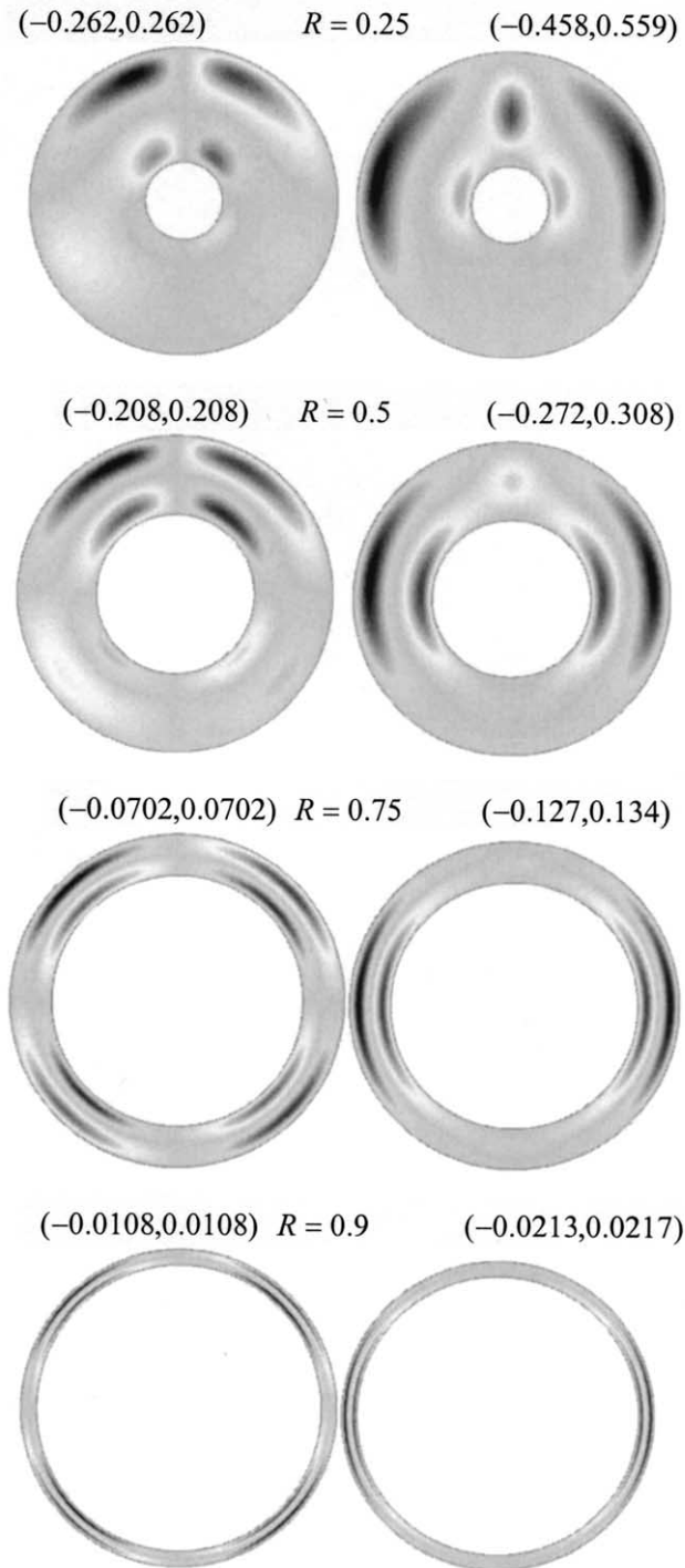
Fig. 11. Effect of the radius ratio on the x-velocity and y-velocity components ( Ra = 10^5 , Pr = 5.49 , N = 1.0 , Le = 0.2 ).
