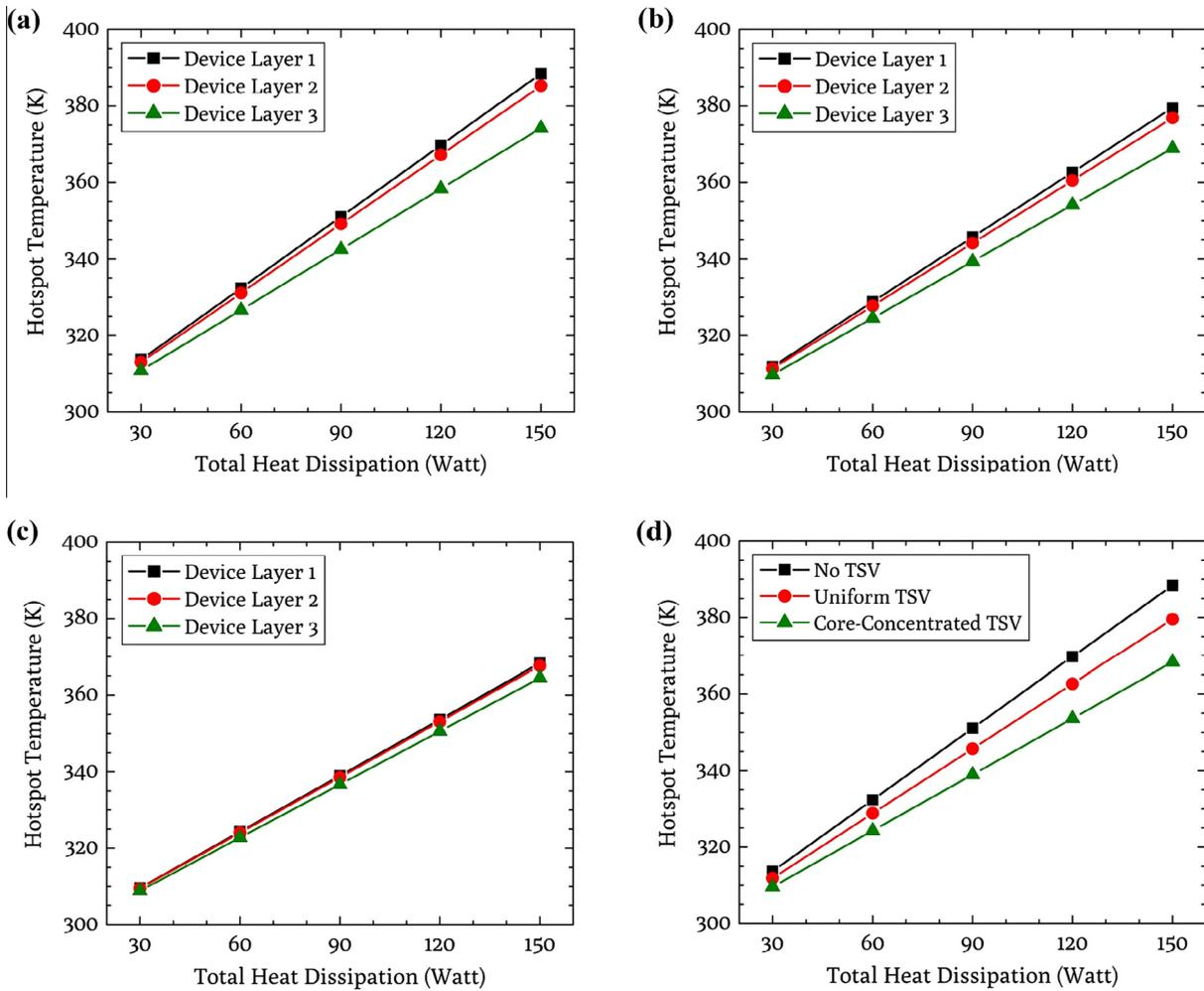
Fig. 10. Effect of the total heat dissipation on the hotspot temperature for (a) No TSV (b) uniform TSV (10% of total chip area) (c) core-concentrated TSV (10% of total chip area) (d) various TSV arrangements (10% of total chip area).
