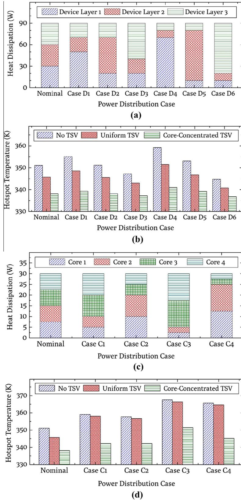
**Fig. 12.** (a) Case study for the power distribution within the device layers (b) effect of the power distribution within the device layers on the hotspot temperatures (c) case study for power distribution within the cores of each device layer (d) effect of the power distribution within the cores of each device layer on the hotspot temperature.
