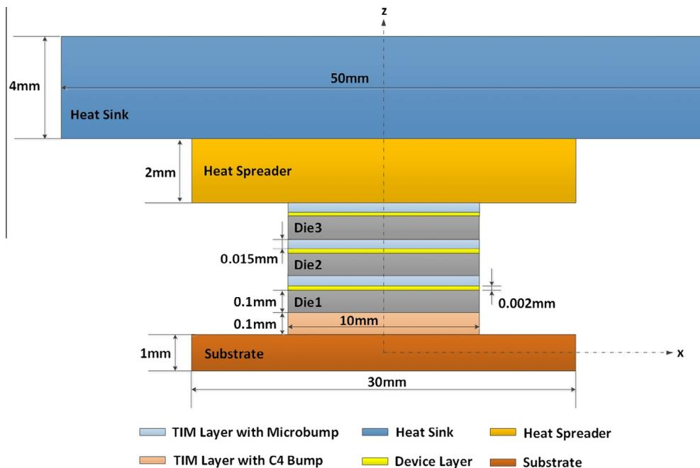
Fig. 1. Schematic of the nominal 3D IC structure.
