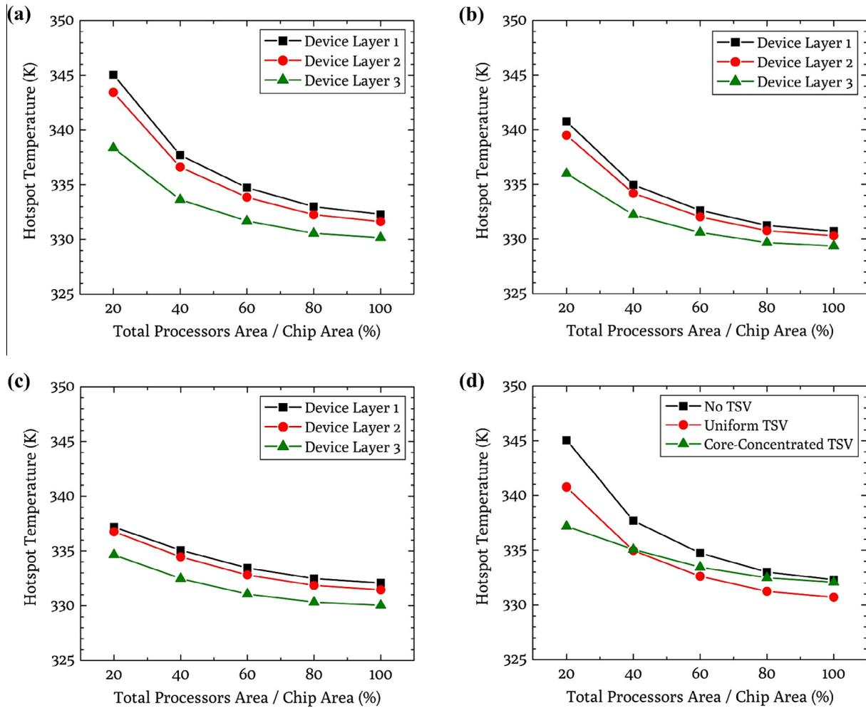
**Fig. 9.** Effect of the processor area on the hotspot temperature for the same chip area and total heat dissipation for (a) No TSV (b) uniform TSV (10% of total chip area) (c) core-concentrated TSV (10% of total chip area) (d) various TSV arrangements (10% of total chip area).
