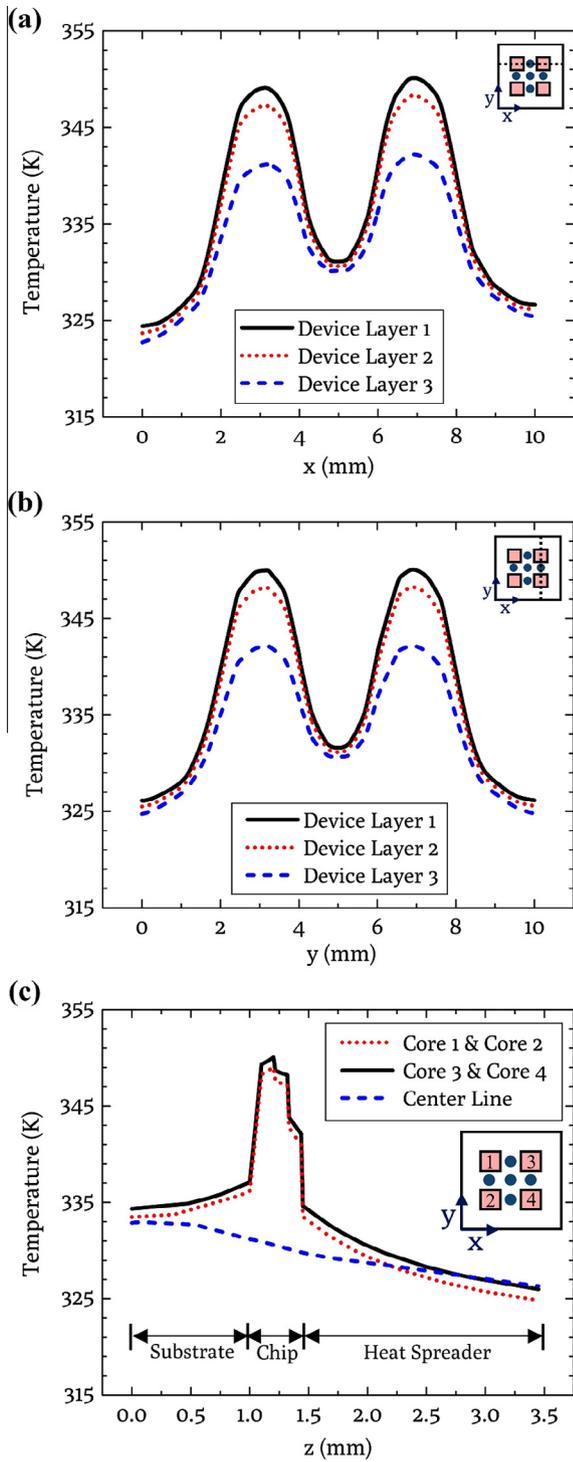
**Fig. 5.** Temperature distribution for the nominal benchmark 3D IC (a) along  $x$  direction for each device layer (b) along  $y$  direction for each device layer (c) along  $z$  direction at the vertical center line of each core and the center line of chip.
