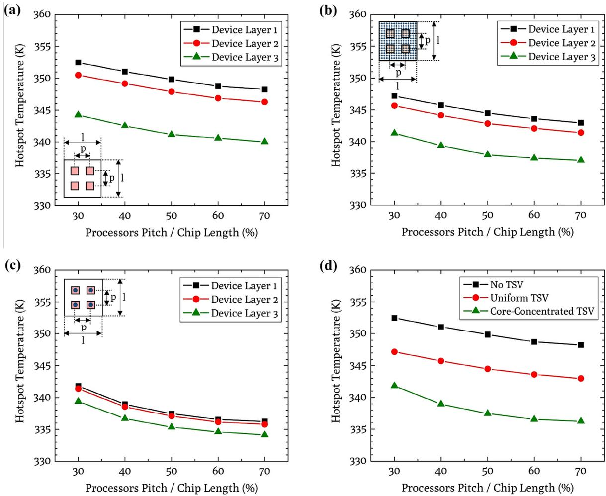
Fig. 8. Effect of processors pitch on the hotspot temperature for (a) No TSV (b) uniform TSV (10% of total chip area) (c) core-concentrated TSV (10% of total chip area) (d) various TSV arrangements (10% of total chip area) for device layer 1.
