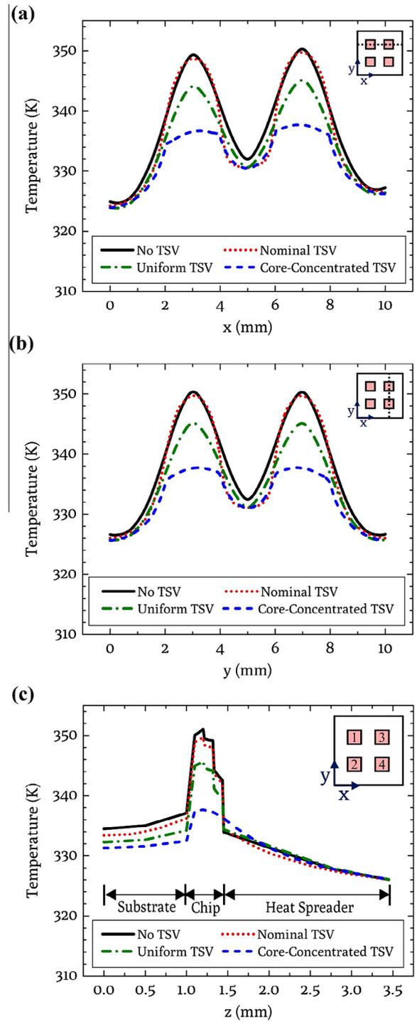
**Fig. 6.** Effect of different TSV arrangement on the temperature distribution of the 3D IC structure (a) along  $x$  direction in device layer 1 (b) along  $y$  direction in device layer 1 (c) along  $z$  direction at vertical center line of core processor 3.
