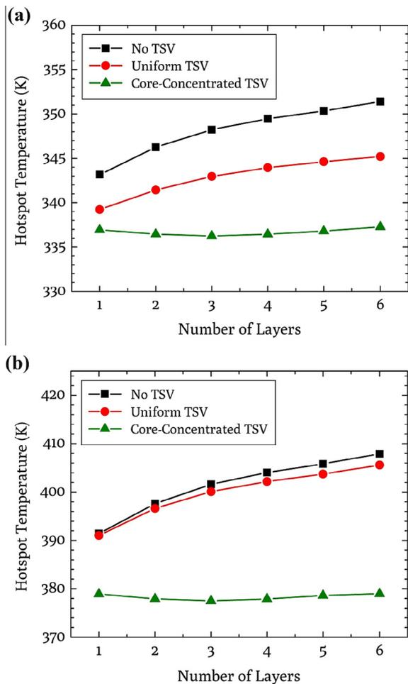
Fig. 14. Effect of the number of layers on the hotspot temperature for (a) 90 W total heat dissipation (b) 180 W total heat dissipation.
