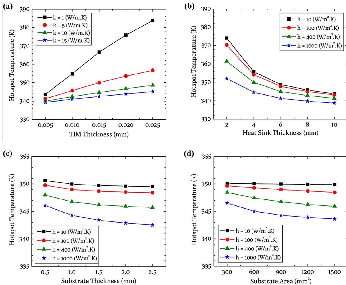
Fig. 11. Alteration of the hotspot temperature through (a) TIM thickness and thermal conductivity (b) heat sink thickness (c) substrate thickness (d) substrate area.
