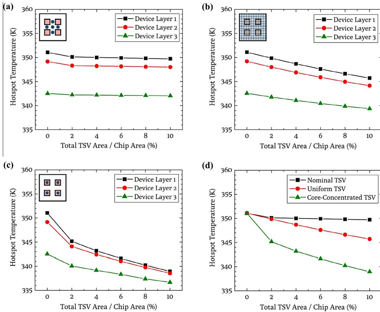
Fig. 7. Effect of the thermal TSV arrangement on the hotspot temperature for (a) nominal TSV (b) uniform TSV (c) core-concentrated TSV (d) various TSV arrangements for device layer 1.
