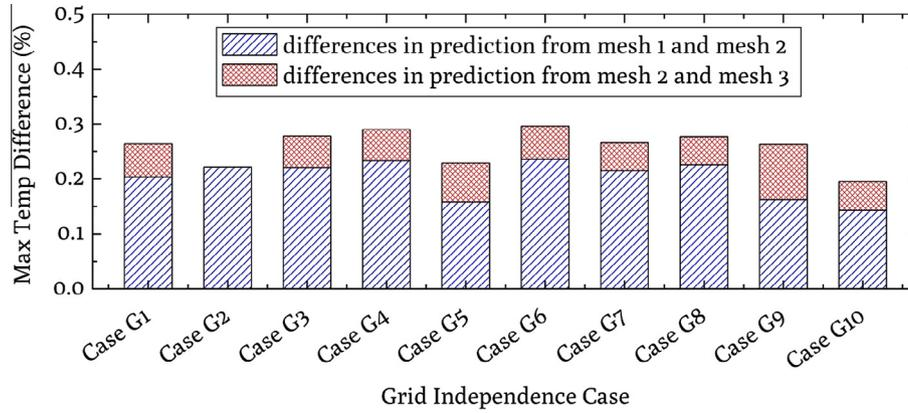
Fig. 4. Grid independence study: the coarsest mesh (mesh 1), finer mesh (mesh 2), and the finest mesh (mesh 3).
