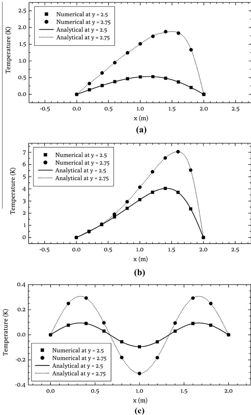
Fig. 2. Comparison with an analytical solution for a slab (a)  $f(x) = 2x$ , (b)  $f(x) = 5x^2$ , (c)  $f(x) = \sin(\frac{2\pi x}{2})$ .
