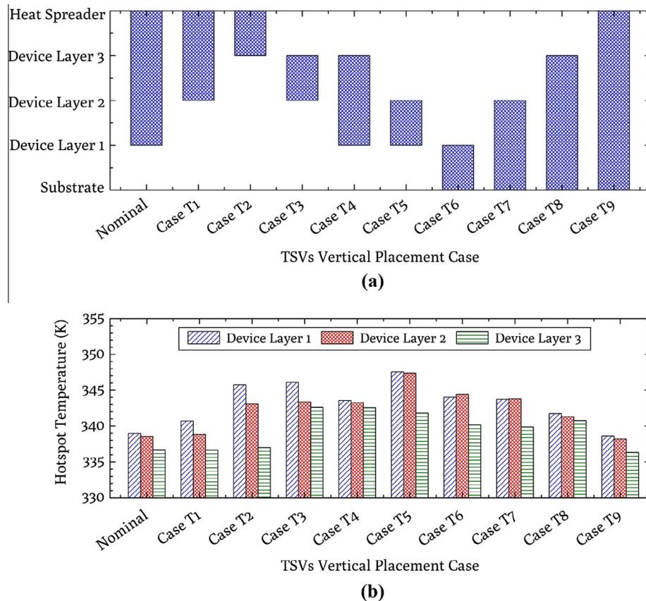
**Fig. 13.** (a) Case study for the vertical placement of the core-concentrated TSVs with a 10% of chip area (b) effect of the vertical placement of the core-concentrated TSVs on the hotspot temperature in each device layer.
