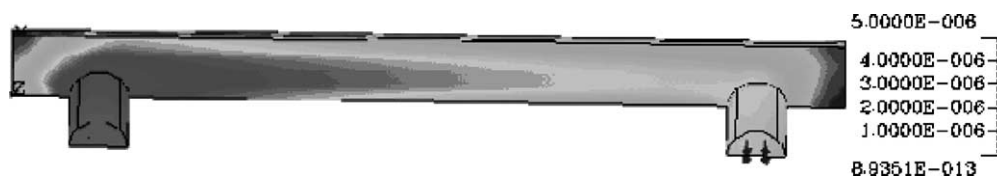
Fig. 3. Distribution of analyte concentration at t = 5 s.
